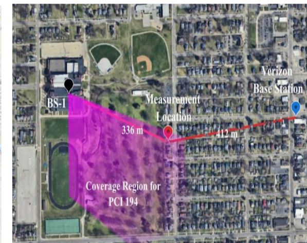
Figure 6: The distance of measurement loc. from the BS-1 and nearby Verizon BS.
