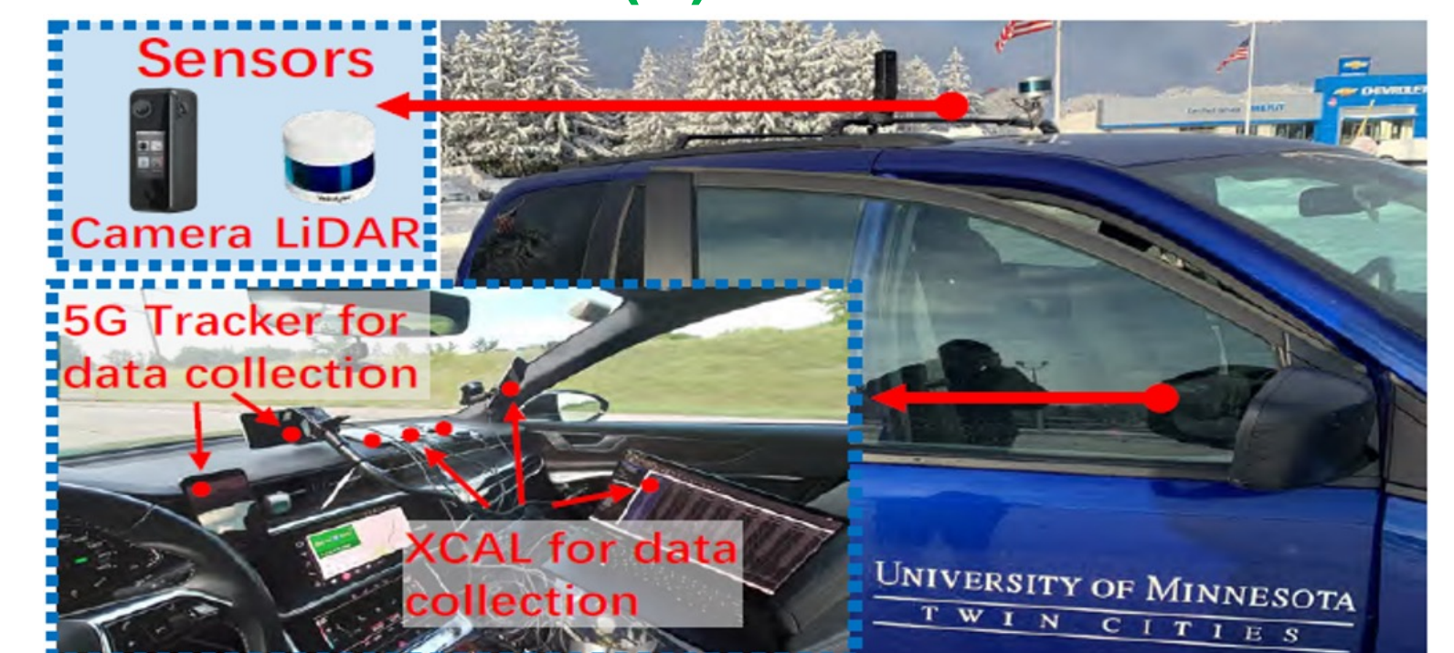
(c) Multi-Modal 5G Measurement Setup
