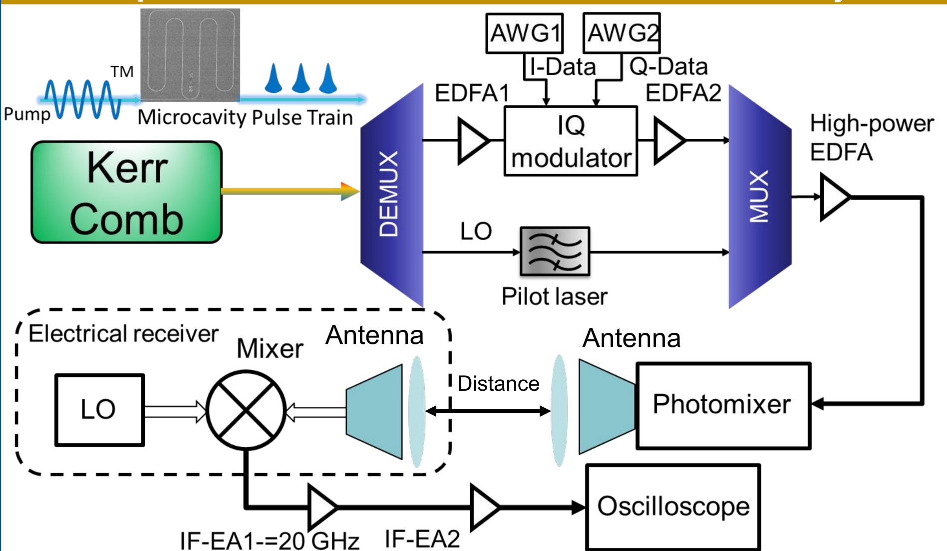
AWG: Arbitrary waveform generator; EDFA: Erbium-doped fiber amplifier; MUX: Multiplexer; DEMUX: Demultiplexer; LO: Local oscillator, EA: Electrical amplifier.
