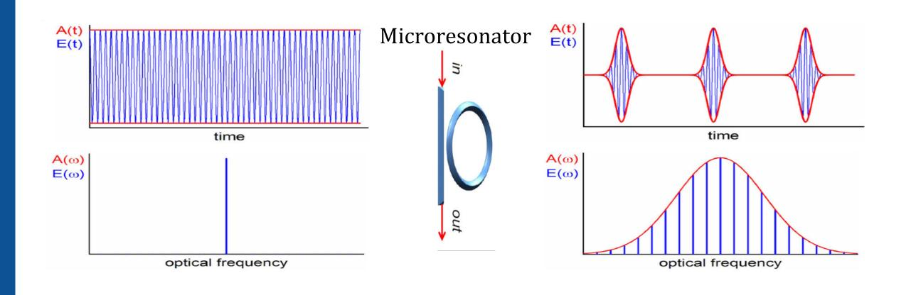
Kerr frequency comb is generated by optical pumping a high-Q microresonator.
