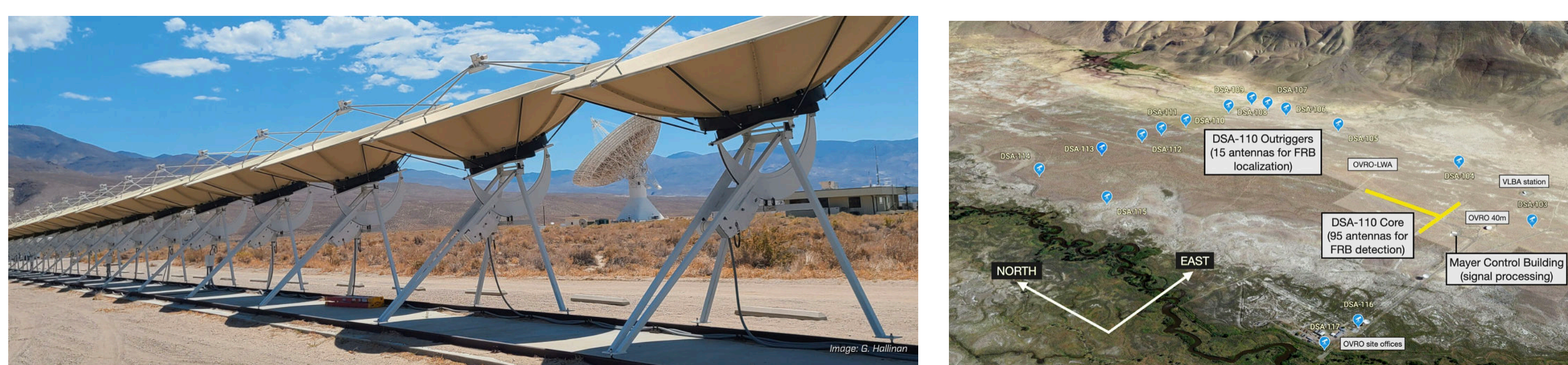
Total 110 dishes, 95 of them are in a Tee-shaped core for searching FRB, with 15 outriggers. Dish diameter - 4.65 m; Frequency band 1280 - 1530 MHz.
